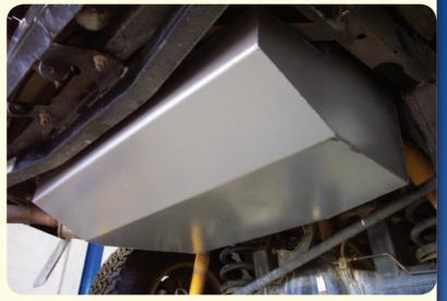
The **M** kit includes everything required to fit the new tank with minimal fuss. The tank is manufactured from 2mm aluminised steel, etch primed and finished in silver hammertone enamel.
