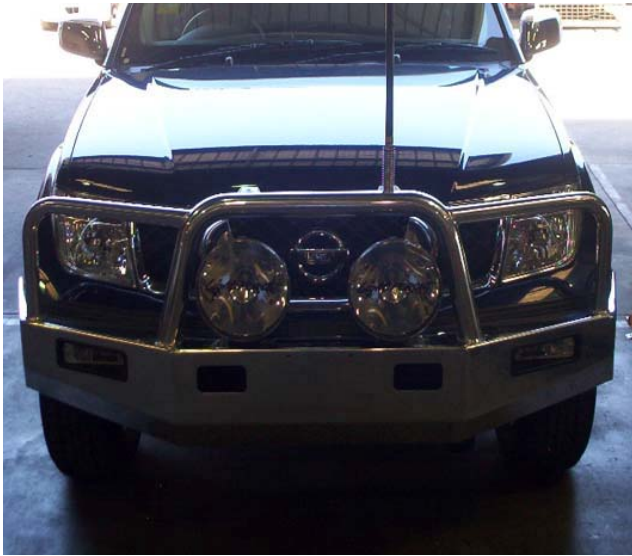
36. Completed fitment of Alloy Bullbar to Nissan Navara.
