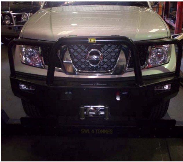
35. Completed fitment of Steel Bullbar to Nissan Pathfinder.
